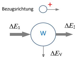
$$\begin{aligned} \sum_{\circ} \Delta E &= 0 \\ (-\Delta E_1) + (+\Delta E_2) + (+\Delta E_V) &= 0 = -\Delta E_1 + \Delta E_2 + \Delta E_V \end{aligned}$$
